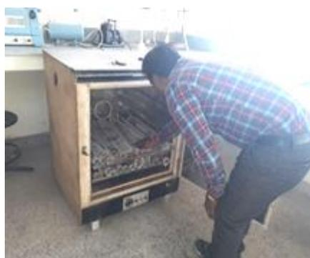
Sample Drying for Dry weight estimation
